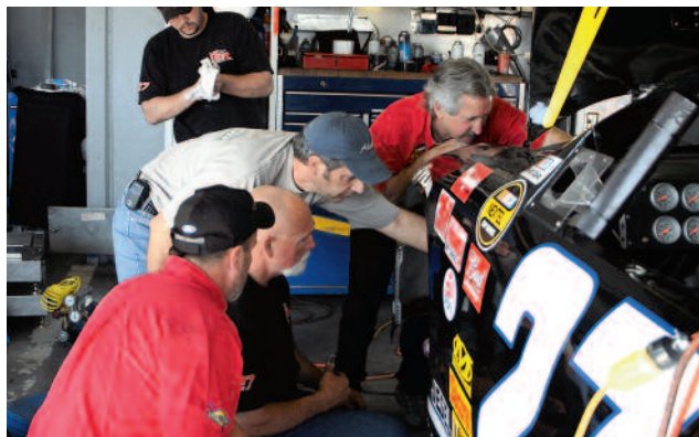
▼ Shelmerdine and his crew check suspension movement after changing the car's upper A-arm. JERRY F. BOONE
