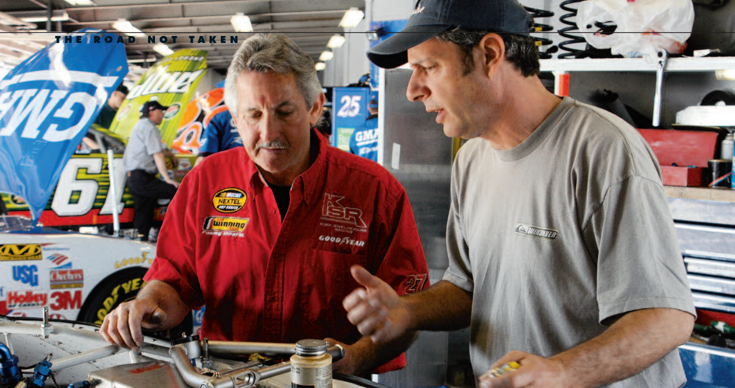
▲ Harris and Shelmerdine discuss replacing the Chevrolet's A-arm with a new piece before the car goes out for its final practice run. JERRY F. BOONE
